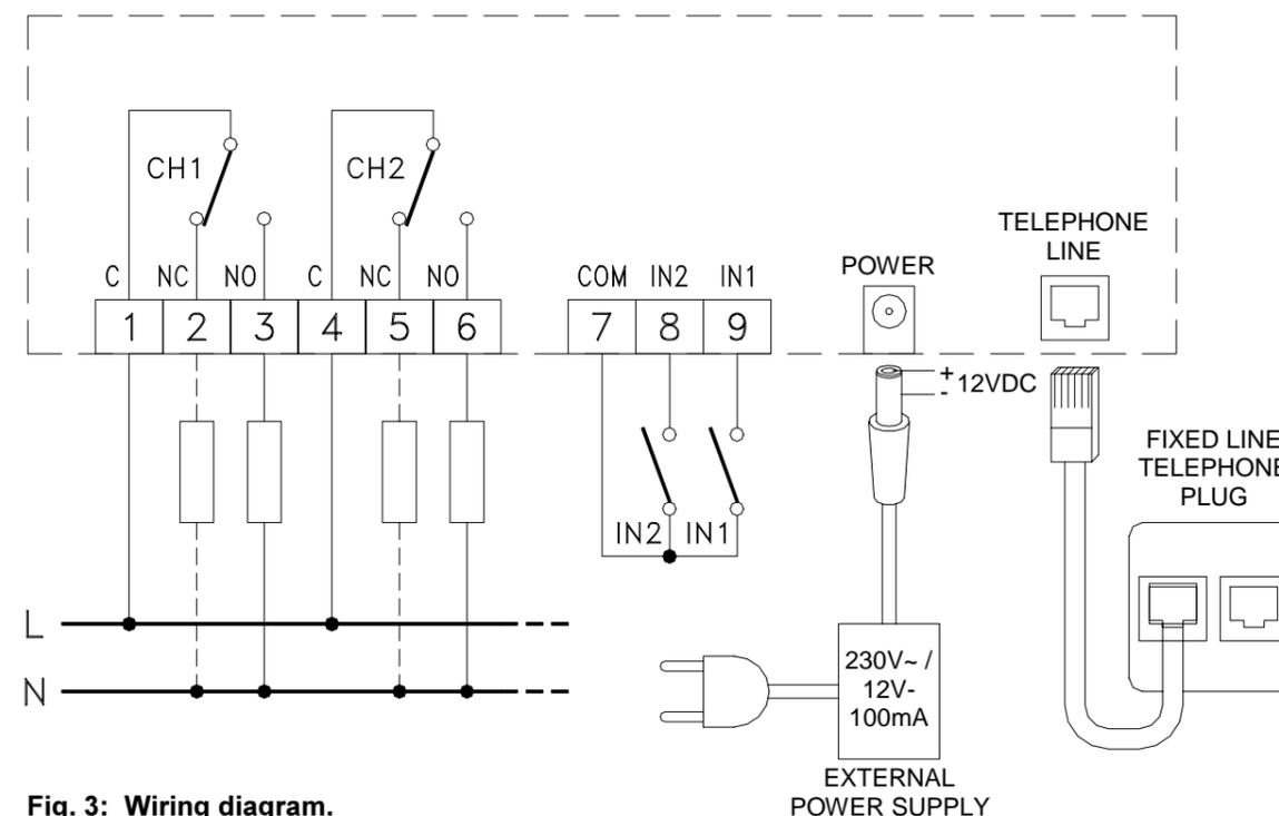
Fig. 3: Wiring diagram.
