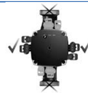
Control box position
