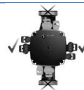
Control box position
