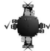
Control box position
